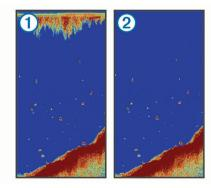
Surface noise ① is caused by interference between the transducer and water. You can hide surface noise ② to help reduce clutter. Wider beam widths (lower frequencies) can show more targets, but can generate more surface noise.
