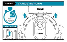
Place robot on dock to charge. The dock indicator light will turn **blue** and the robot will beep when charging begins.
