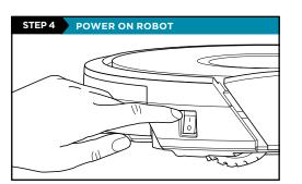
To charge, the **Power** button on the side of the robot must be in the ON position (I).
