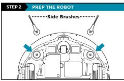
Remove protective film from robot and dock. Attach side brushes.
