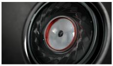
The 50 mm acoustic drivers boast diaphragms composed of multiple polymer layers, and filled with damping gel. The flexibility and smoothness of each diaphragm delivers perfectly balanced sound. The bass is impactful without being overpowering. Midrange frequencies are full and smooth. High frequencies are exquisitely detailed.
