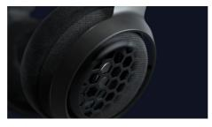
The open-back ear-cup design is covered with acoustically transparent Kvadrat speaker fabric. Air is able to flow freely through the fabric-eliminating air pressure build-up behind the diaphragm and creating immersive, spacious sound.
