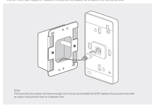
4. Attach the EAP to the mounting bracket by aligning the two mounting studs on the mounting bracket with the large openning of the slots on the EAP. Press and slide the EAP down until it
