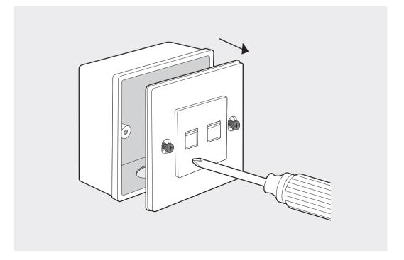
2. Insert the enclosed screws and tighten them with a Philips screwdriver to secure the mounting bracket.
