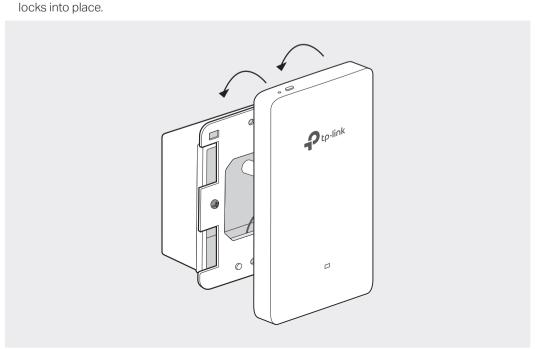
To remove the EAP from the mounting bracket, insert a paper clip into the hole next to the LED button to release the Locking Tab. Slide the EAP upwards and pull it out to detach it from the mounting bracket, as shown below.
