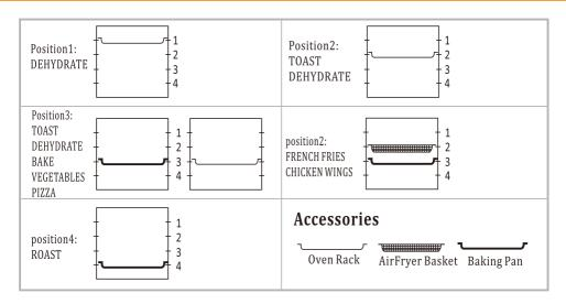
**Note:** When cooking fatty foods (e.g. chicken wings) with the oven rack or the air fryer basket, place the baking pan in the slot underneath in order to prevent oil from dripping on to the stainless-steel heater.
