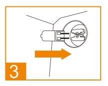
2. Remove the used bulb by pulling it directly.
