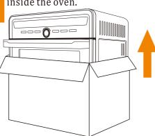
Place on a stable, level, heat-resistant surface, away from anything that can be damaged by heat. Keep at least 110mm(4.33") distance between the electrical outlet and the wall, furniture, etc.
