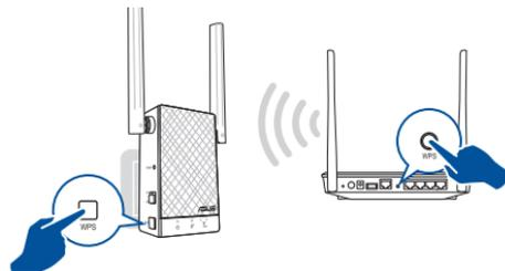
3. Check if RP-AC55's Wi-Fi indicator turns solid light, which indicates that the Repeater has connected to the wireless network successfully. The Repeater's wireless network name (SSID) changes to your existing Wi-Fi network name, ending with **\_RPT** or **\_RPT5G**. For example:
