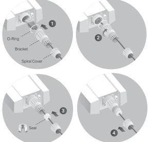
Fit an Ethernet cable through the Spiral Cover, Bracket, and O-Ring, and connect the cable to the port.
