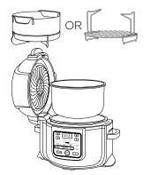
2 Follow the instructions on page 15 to install the pressure lid. Turn the pressure release valve to the VENT position.
