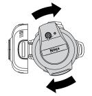
**3** Make sure the pressure release valve on the lid is in the SEAL position.
